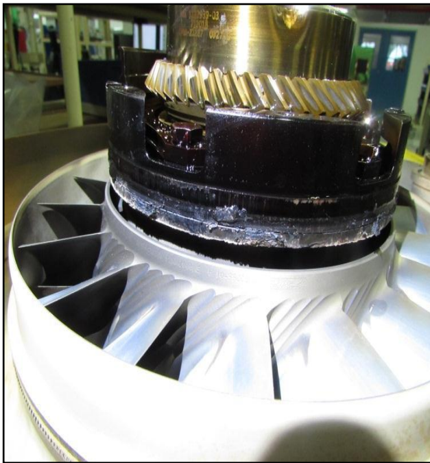
DETERIORATED PACKING OF NO. 4 BEARING HOUSING
