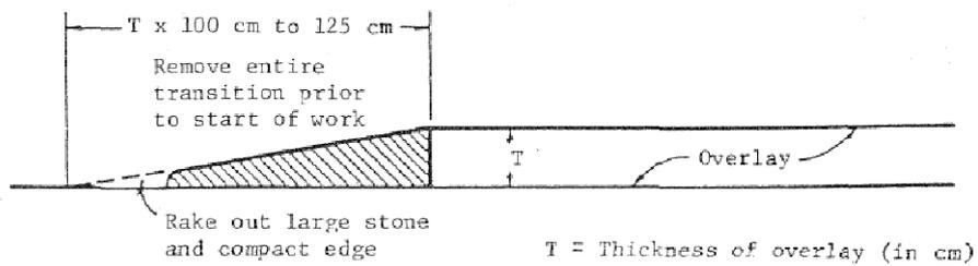
**Figure-C** Temporary ramp construction without cold planing machine
