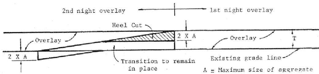
**Figure-B** Temporary ramp construction with cold planing machine
